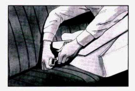
Pick up the latch plate, and run the lap and shoulder portions of the vehicle's safety belt through or around the restraint. The child restraint instructions will show you how. Tilt the latch plate to adjust the belt if needed. If the shoulder belt goes in front of the child's face or neck, put it behind the child restraint.
